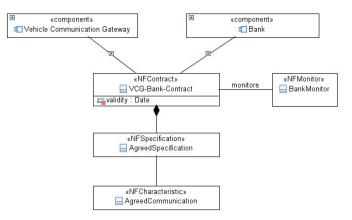
Figure 21: Contracts between the Vehicle Communication Gateway and the Bank components
