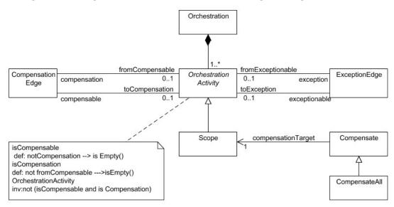
Figure 5: UML4SOA metamodel: package Behaviour - Compensation
