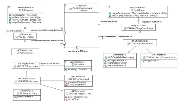
Figure 20: Specifications of non-functional properties for the Vehicle Communication Gateway
