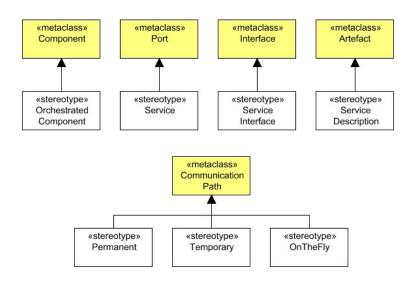
Figure 9: UML profile for service-oriented systems: structural elements
