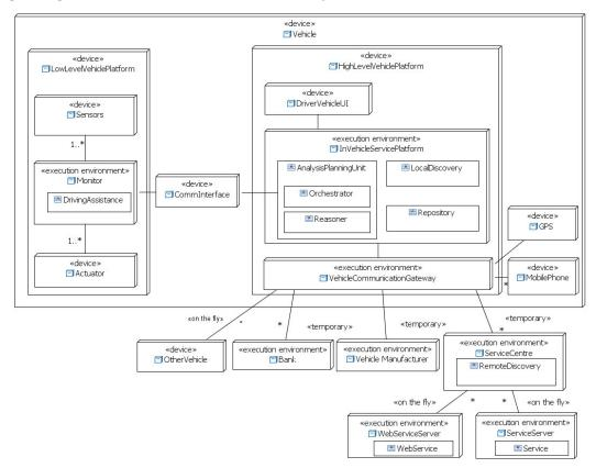
Figure 15: UML deployment diagram for the Architecture of the automotive case study
