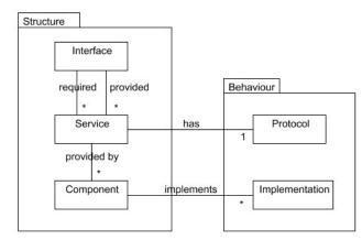
Figure 1: Main concepts in the Service-Oriented Architecture Profile (UML4SOA)
