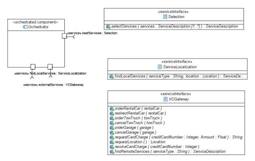
Figure 16: UML structure diagram for the Orchestrator component in the On Road Assistance scenario
