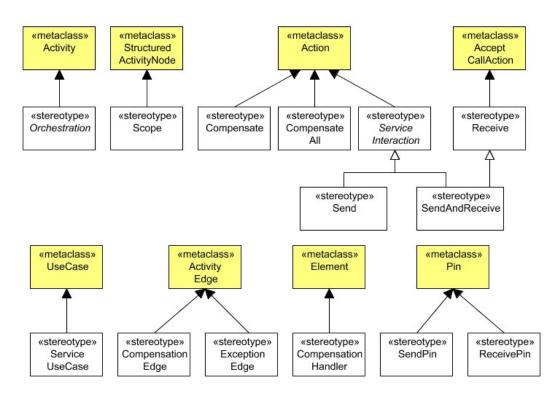
Figure 10: UML profile for service-oriented systems: behavioural elements
