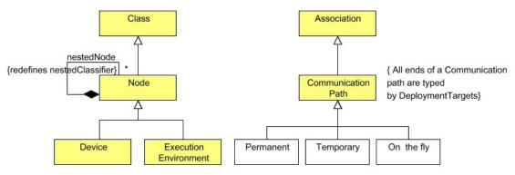
Figure 3: Deployment: (a) UML model elements (b) UML4SOA metamodel: package Structure
