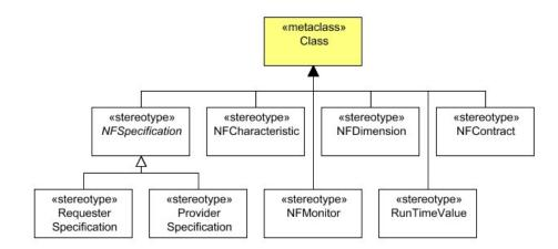
Figure 13: UML profile for service-oriented systems: Non-functional properties
