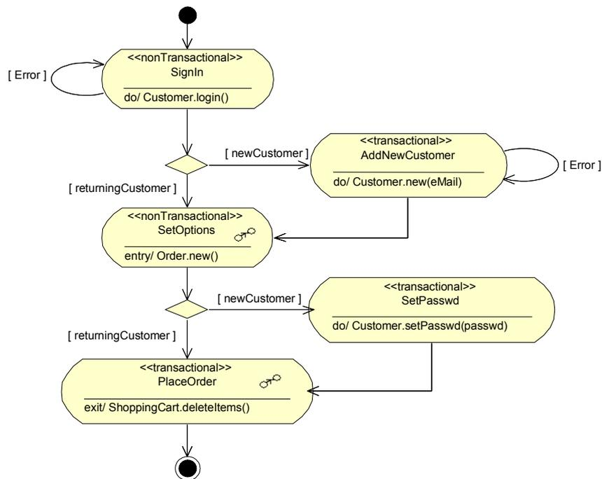
Figure 6. OO-H Refined Activity Diagram of the Checkout Process in [www.amazon.com](http://www.amazon.com)
