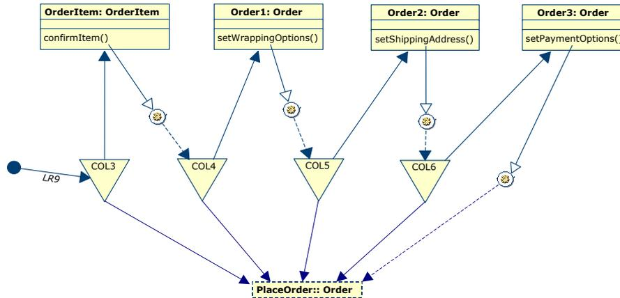
Figure 8. NAD Diagram Corresponding to the *SetOptions* Subactivity State
