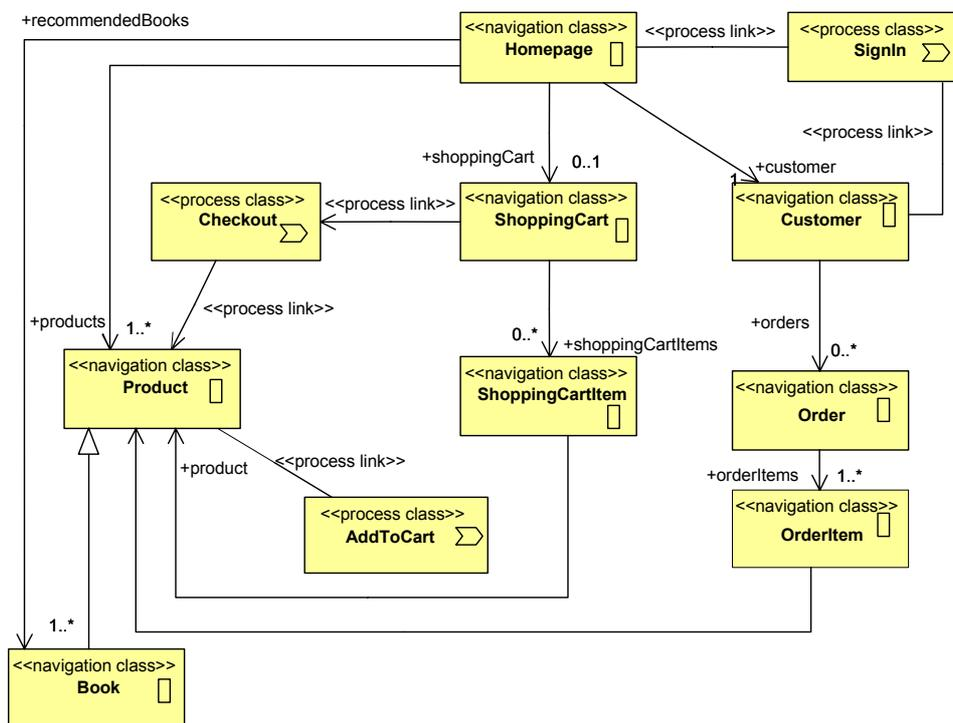
Figure 9. UWE Navigation Model of the Checkout Process in [www.amazon.com](http://www.amazon.com) (First Step)
