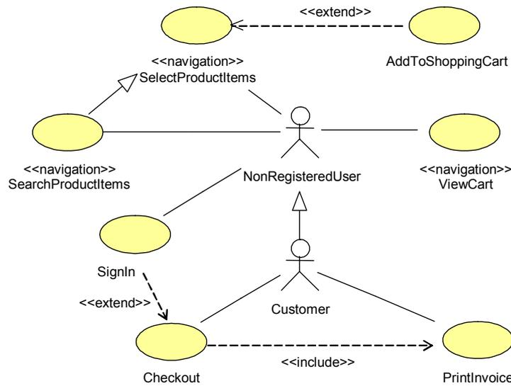
Figure 1. Use Case Diagram of the Checkout Process in [www.amazon.com](http://www.amazon.com)
