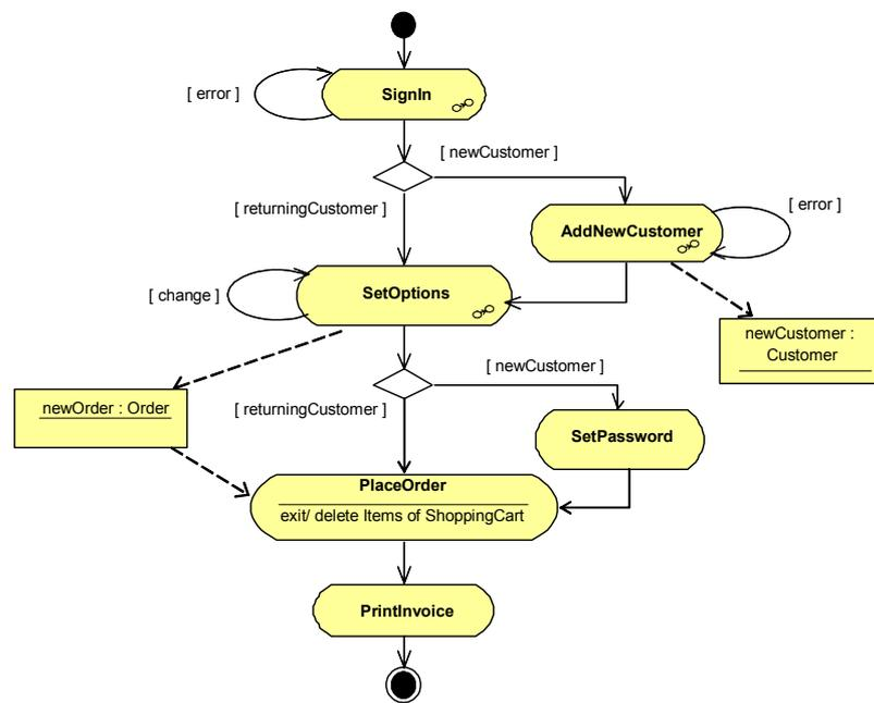
Figure 3. Process Model of the Checkout Process in [www.amazon.com](http://www.amazon.com)
