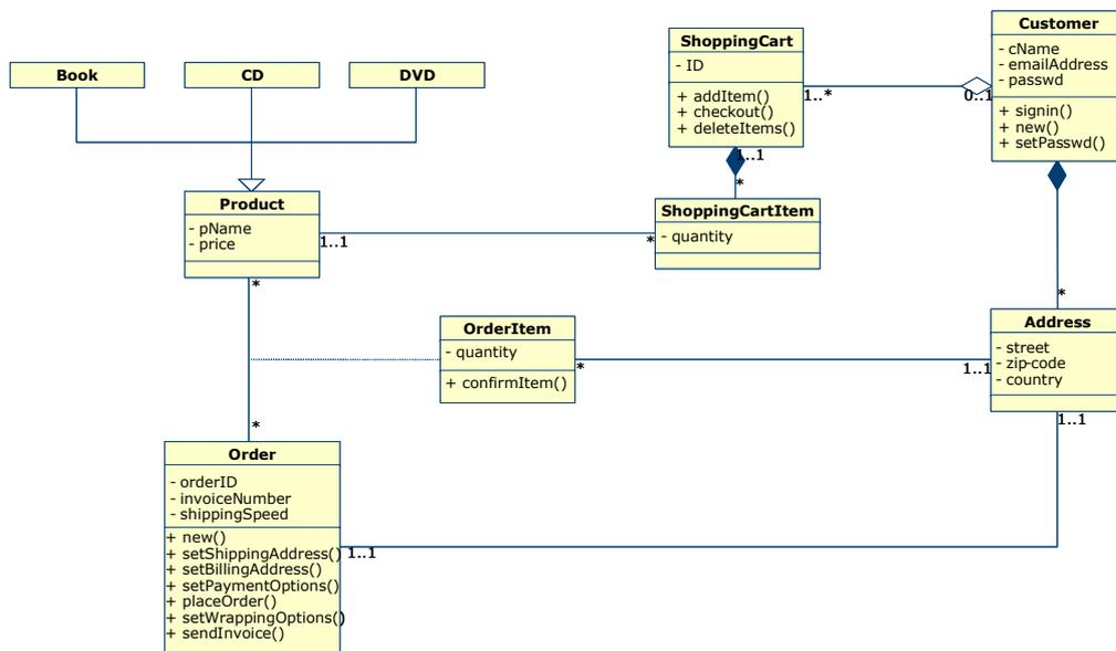
Figure 5. OO-H Refined Class Diagram of the Checkout Process in [www.amazon.com](http://www.amazon.com)
